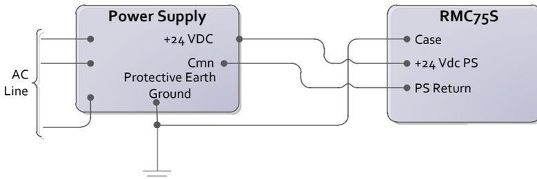
Tighten the wire clamp screws on the terminal blocks to 7 lb-in (0.8 Nm).
