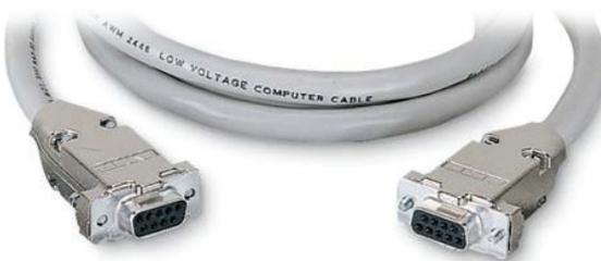
If you make your own cable, pins 2 and 3 must be crossed over, and pin 5 must be straight-through.
