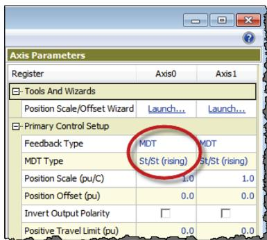
2. Set the **MDT Type** register to the type of MDT transducer you have. This information is available on the transducer datasheet.
