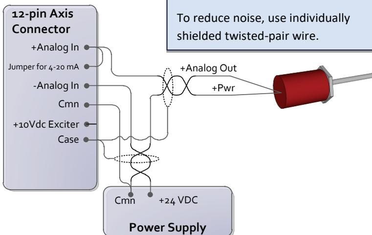
The **Jmpr** and **-In** pins are internally connected via a 250Ω resistor.
