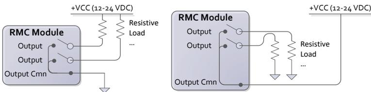
When switching *inductive* loads, place a diode or transistor across the load to protect the switch when it turns off. Otherwise, a voltage spike in excess of the 30V rating of the SSR may occur. See the **D8 Wiring** topic in the RMCTools help for more details.
