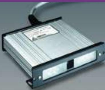
Twenty-eight high-intensity LEDs, along with a precision photodetector, form the core of the CS64A color detection system. The unit determines color by turning on the LEDs—one color at a time—and analyzing the diffuse reflected light from the material or object in the sensing area.
