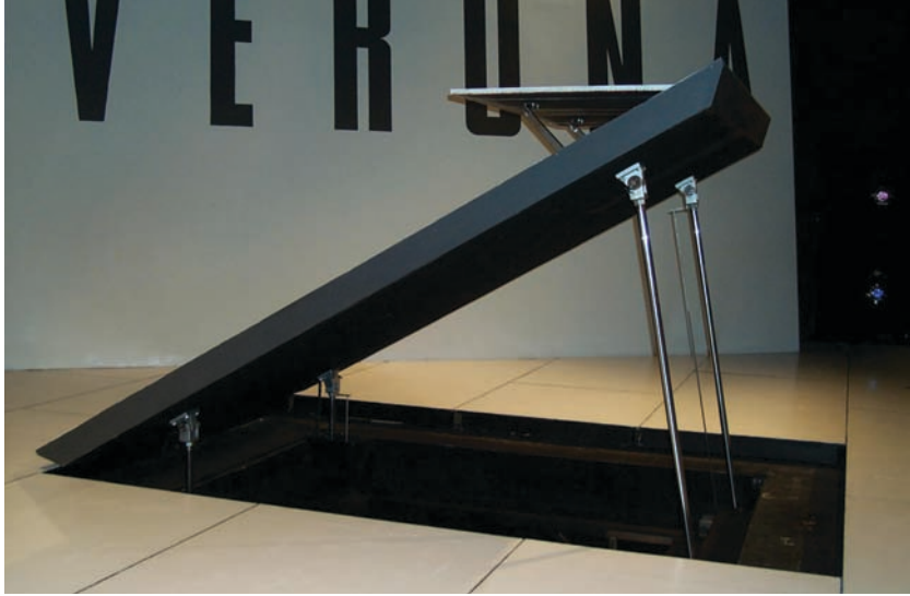
The hydraulic platform extended in position as Juliet's balcony. The small electrically-driven "anti-rake" platform is visible at the top of the main platform.
