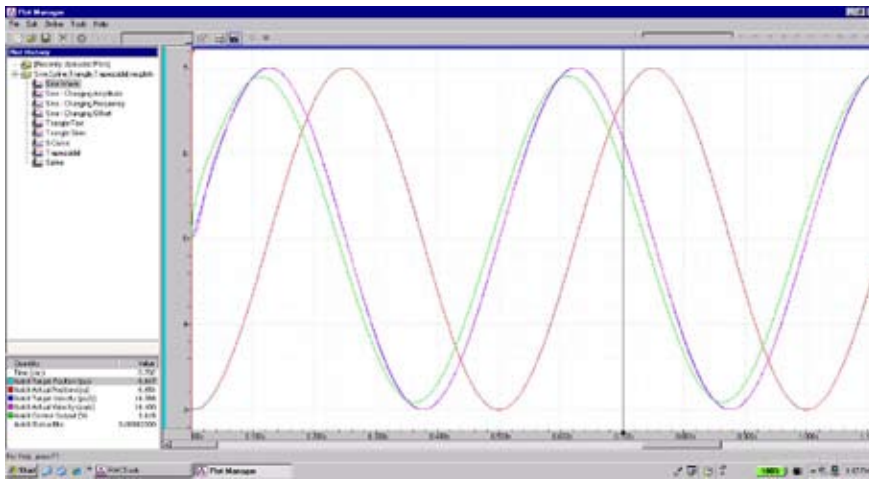
Figure 2a. A plot of continuous sinusoidal motion produced by an RMC150 motion controller. The red curve plots axis position versus time and the violet curve plots velocity versus time. As this system is tuned precisely, the actual and target position and velocity curves overlap.
