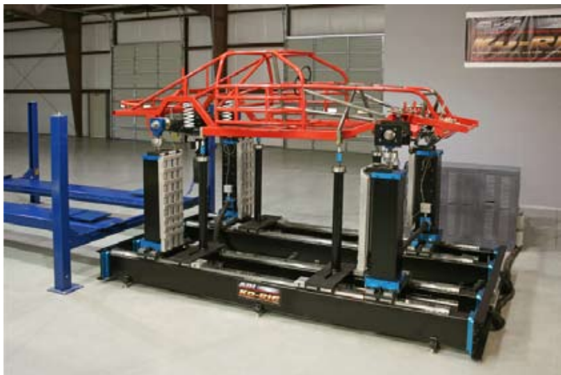
Figure 5. Vehicle suspension test system.
